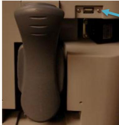
The USB network adaptor is inserted here, behind the cover panel. The USB will flash blue if it is connected
