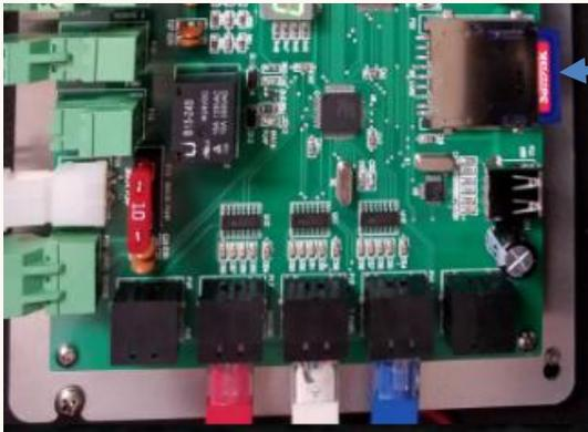
Location of SD card slot- accessible from an external access hatch.
