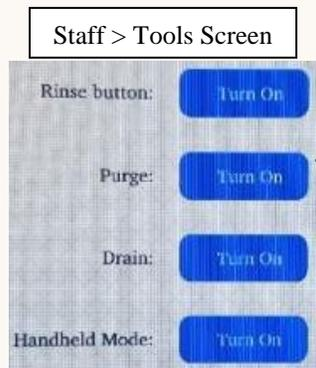
**Note:** The default purge time is 90 seconds. This should be sufficient to purge the lines.
