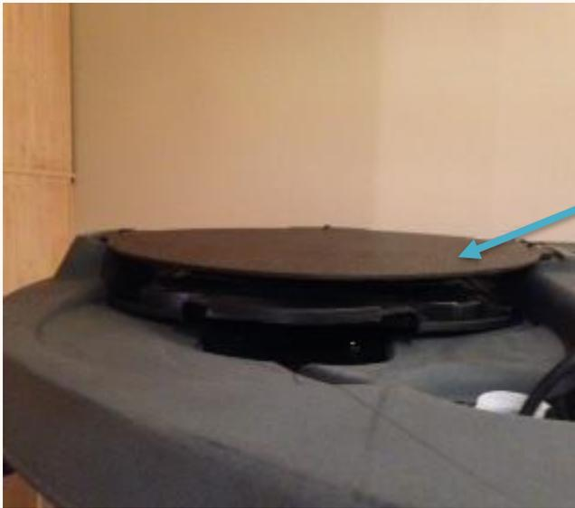
The **top exhaust filter** is located on the ceiling of the booth (upper left side if facing the booth). Please use a stepladder to reach safely. **Follow all directions on the ladder to avoid a fall.**
