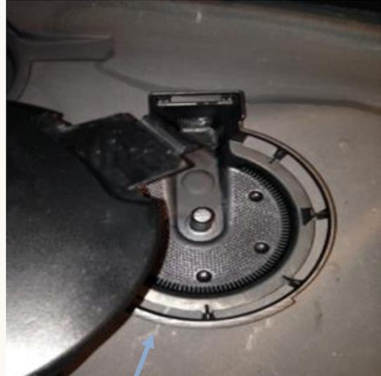
The cover will snap off easily (do not apply excessive force). Remove the filter and wash in sink to dispel any sediment that may have accumulated from bodies or surfaces. You may need a soft bristled brush to brush away lint or sediments from the filter. Clean the sump basin of any sediment, then replace the filter and slide the cover back into place. Now, move to the touchscreen.
