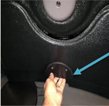
Carefully remove the bottom panel by pulling out on the handle. If the panel has an accumulation of solution, clean with warm water and Dawn or other mild detergent.
