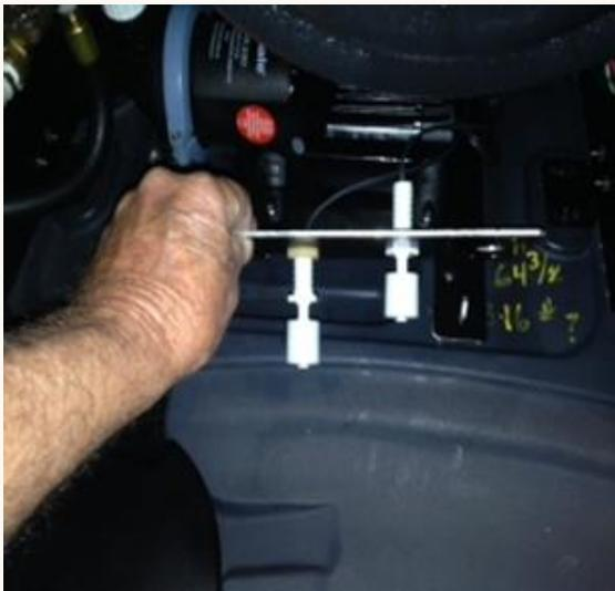
Being careful **not to damage the float sensors** in any way, lift up the float switch plate and **carefully** clean both floats. Do not use excessive force on the floats.
