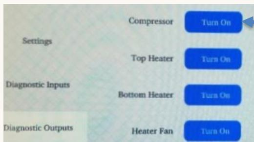
Press the Turn On button for the compressor and check the specs displayed to the right. The PSI value is ideally 19.5 PSI, but in the range of 18.5 to 20.5 is acceptable. See Appendix 2 for more on tolerances.
