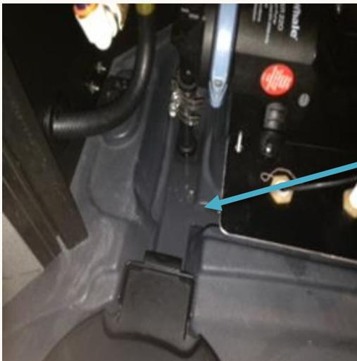
Clean the sump basin and remove any debris. Use a nonabrasive cloth and warm water to clear any sediment that may have accumulated.
