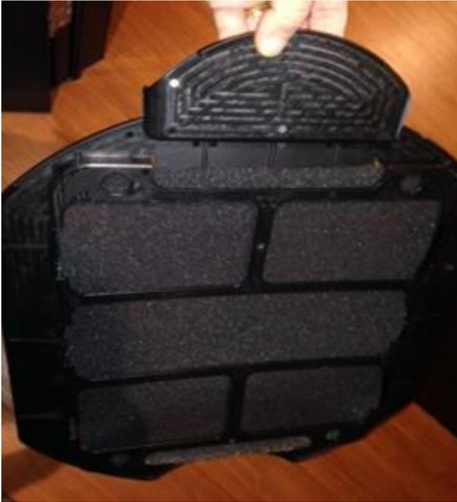
Once the top exhaust filter is removed, take it to a sink and wash with warm water. Only once the filter has been allowed to **fully dry** should it be reinserted into the ceiling. Do not run the booth with the top exhaust filter removed.
