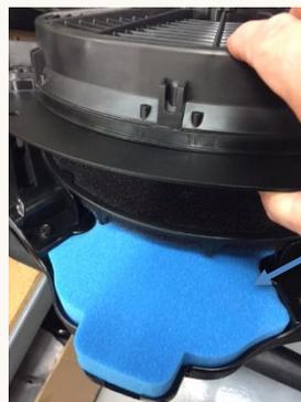
4. Remove and clean the smaller blue filter, using warm water and replace with the spare filter while drying.
