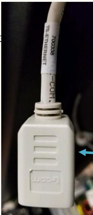
Image of the female Ethernet connection for the booth. Use a male cable with CAT 5 or better (CAT 6 is compatible).
