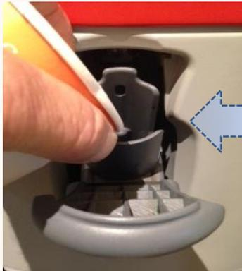
Open the cartridge receptacle pour in ¼ cup of warm clean water into the reservoir. On the touchscreen, go to Staff > Tools and select Purge. Inspect the air pressure value displayed. If the value is not in the range of 18.3 – 20 PSI see T5. Adjusting Air Pressure.
