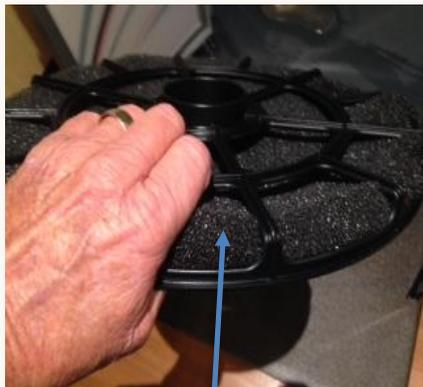
2. Remove the existing filter and clean, using warm water. Have spare filter on-hand.
