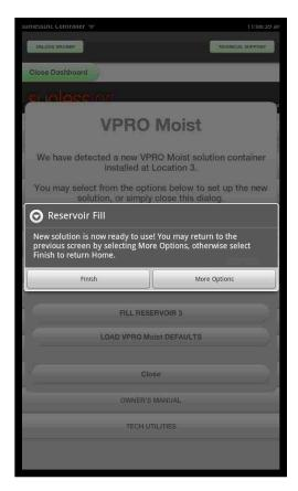
6. After selecting the More Options button in the previous step, change the number of Purge Cycles to 4 in the following screen, then select the Purge button to continue. This will now pump the new solution through the lines and to the nozzles.
